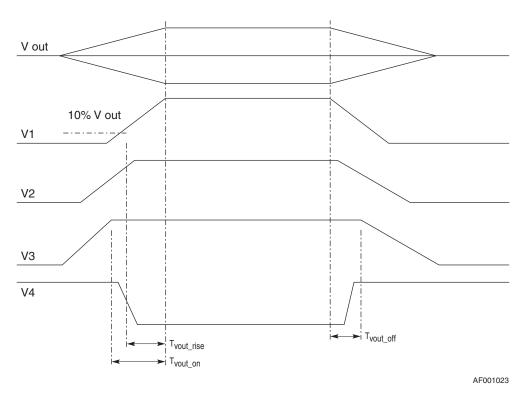
Figure 12. Output Voltage Timing
