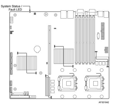
Figure 9. System Status / Fault LED Location
