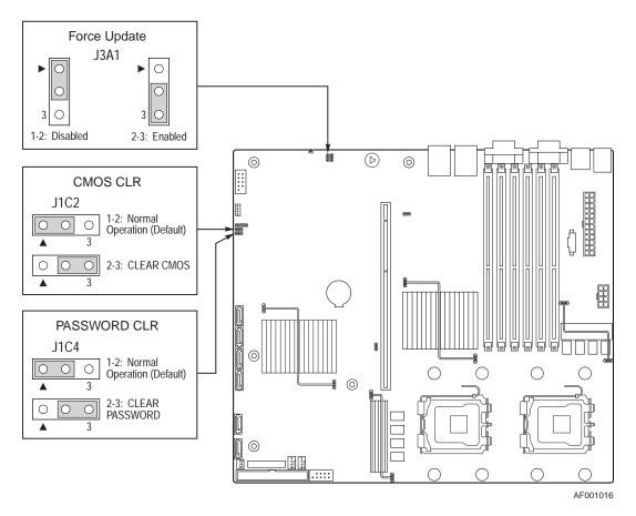
Figure 8. Recovery Jumper Blocks (J3A1, J1C2, J1C4)
