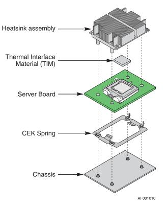
Figure 5. CEK Processor Mounting
