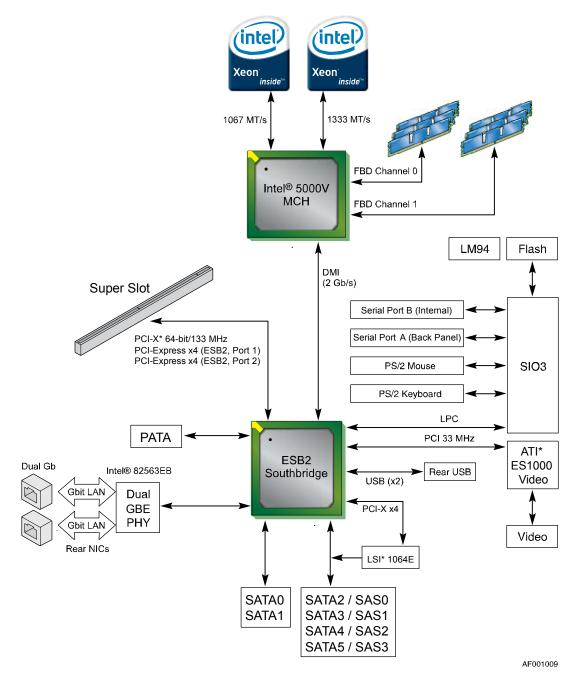
Figure 4. Functional Block Diagram
