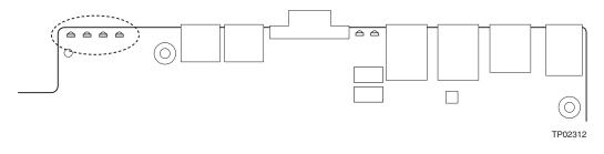
Figure 11. POST Code Diagnostic LED Location
