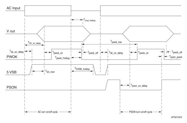
Figure 13. Turn On/Off Timing (Power Supply Signals)
